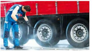
This optional extra allows the user to manually improve the automatic wash with a high-pressure gun working at **160 bar** and with **18 L/min**. Using the same gun, shampoo can be applied together with the high-pressure, and a 15 bar chemical pre-wash program can be selected. The external control panel can be mounted at a distance or wall-mounted. A reel can be installed too. The unit can work with hot water and with softened water.
