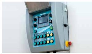
This optional external command post with a colour touch-screen facilitates **navigation** on the machine menu. It consists of selector switches to turn on and off the vertical and horizontal brushes, push buttons to manually move the machine and the brushes, and program selection push buttons (up to 14 pre-set programs).
