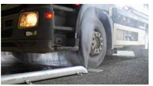
Drive-through underchassis wash with high-pressure system, 70 bar and 126 L/min. With entry photocells for an automatic operation and 12 rotating zero-angle nozzles. Can be supplied from the same high-pressure pump rack as the lower side high-pressure optional extra by means of a solenoid valve.
